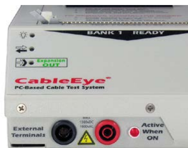
External Terminals for Chassis and Component Testing
