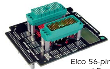
Adapter Cables for a Complex Four-Board Harness Interface
