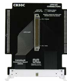
CB30C Molex 160-Pin LFH Connectors (Item 760C)
