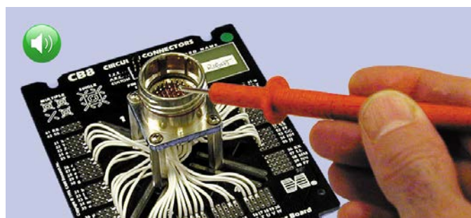
Using the Probe when Making a Pin Map
