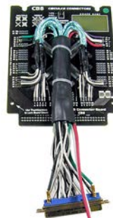
Adapter Cable and Flying Leads for Automotive Harness
