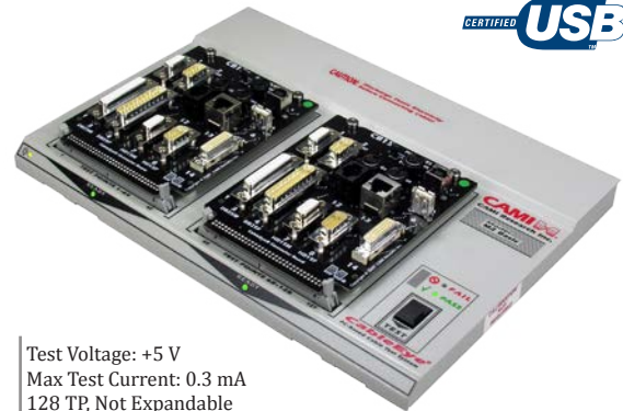
CableEye M2U-Basic (Item 810U) with CB15 Boards (Item 745) Installed
