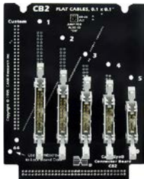
CB2 (Item 732) Large and Small Dual-Row Headers for IDC Flat Cables
