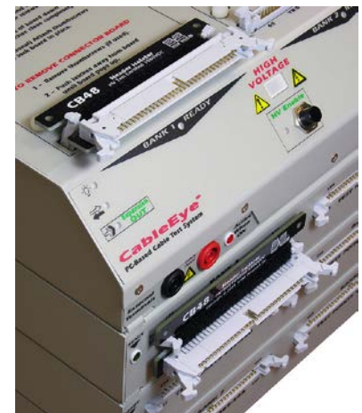
CB48 A (Front) and B (Top) Installed on an HVX Tester. Use for M3U-series testers too.
