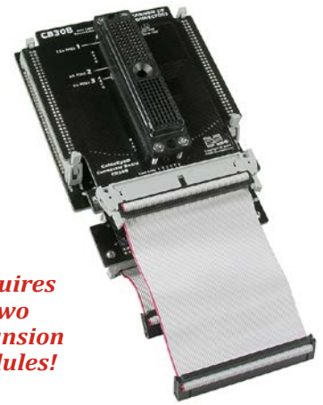
Top View of CB30B (Item 760B) Mounted on CB30 (Item 760)
